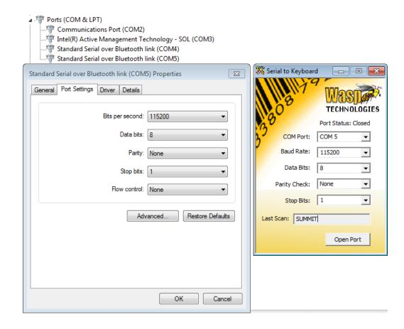
If you still encounter problems with getting an SPP mode scanner communicating to Windows, there are several registry settings that can be cleared. Remove the paired scanner, clear the registry entries, then try the pairing process again.
