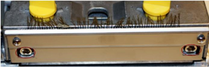
The print head burn line adjustment knobs are used to fine tune the print quality for different thickness of media. Turning the knobs adjusts the print head's burn line forward or backward as it relates to the platen roller.
