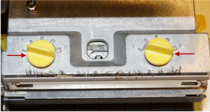
Because the printer's paper alignment is to the left side of mechanism, different media widths require different pressure to print correctly.
