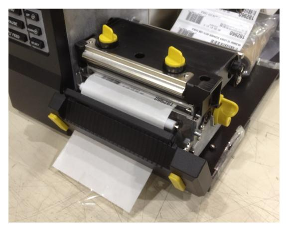
Then close the cover. When labels feed out at print time, the backing will continue down through the slot as the peeled labels are presented to the user above.
