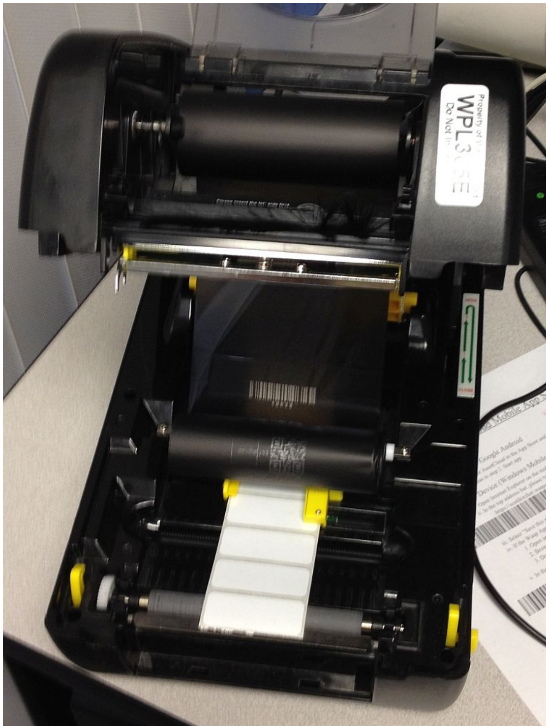
Loading the ribbon (side view). Pull the used/takeup spindle forward, then up, and mount it at the front. Wind up any slack by rotating the spindle clockwise (viewing the printer from the right).
