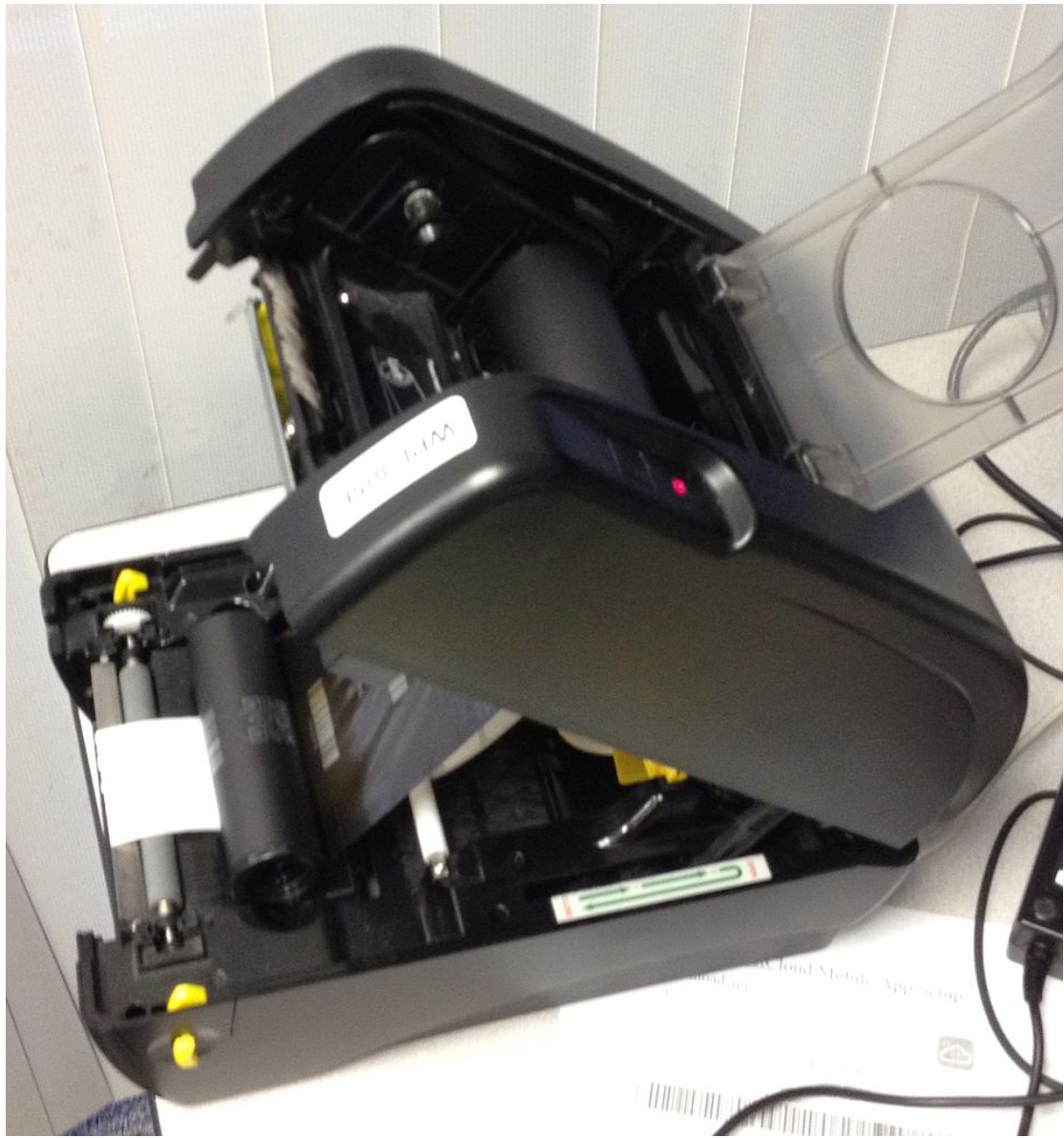
This shows the ribbon loaded properly. The unused supply roll is in back, and the used takeup roll is in front. The dull side is what shows here; this is the ink side of the ribbon. The shiny side does not have ink on it.
