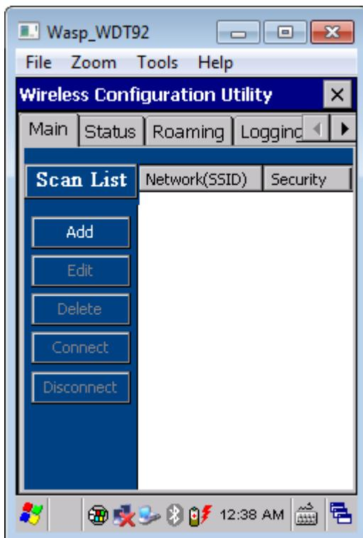
Main tab, tap Scan List button to get a list of advertised networks (SSIDs). Optionally, tap the Add button instead to manually specify the network name, encryption type, etc.
