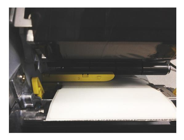
If the printer will not successfully auto-calibrate, it's possible there is paper debris or a stuck label blocking the sensor. You may be able to clear paper debris with blast(s) of compressed air. It may also be necessary to closely examine the sensor and manually remove obstructions.
