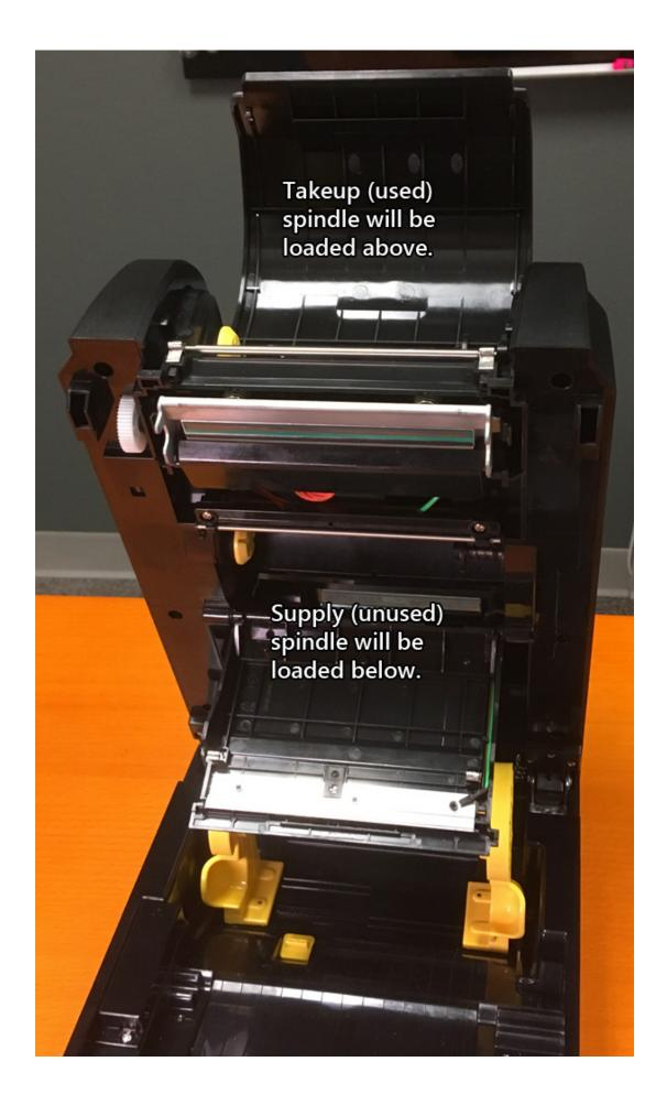
4. Leaving the takeup (used) spindle below, pull the supply (unused) spindle up, then slide it in and to the right, engaging the right/black side of the spindle to the black spring-loaded hub. Then slide the left/yellow side onto the yellow hub. The yellow tabs should engage the yellow slots.
