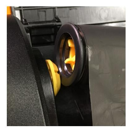
6. Roll the left side of the takeup spindle forward/counter-clockwise to tighten the ribbon.
