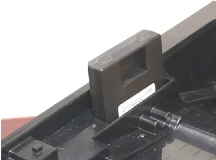
Push the module down until the module connects to the internal connector. The picture below shows the module fully inserted.
