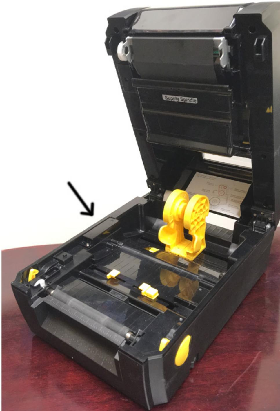
Use a #2 or #3 Phillips screwdriver to remove the screw.
