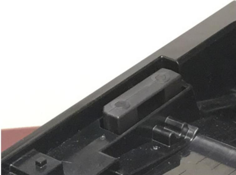
Replace the module cover and put the screw back in. Tighten snugly but not too tight, since the housing is soft plastic.
