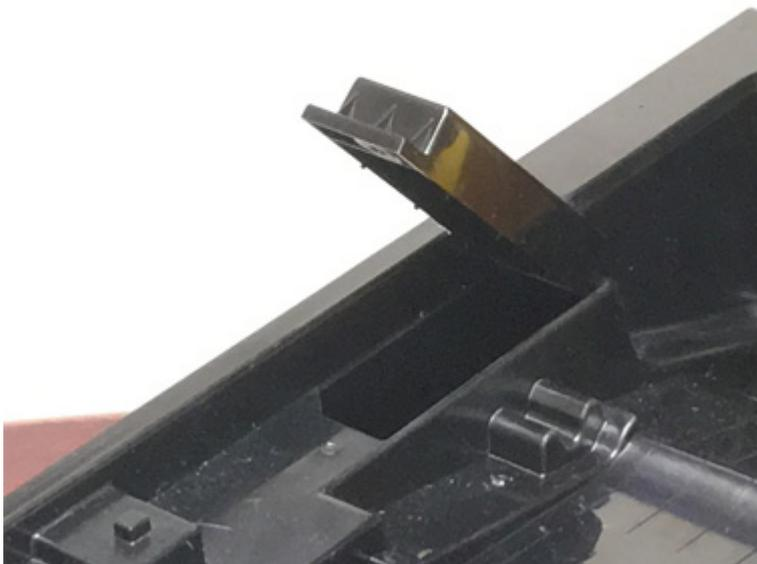
Orient the module so the diagonal corner matches the opening, and the 10-pin connector points down. Insert the module firmly but gently.
