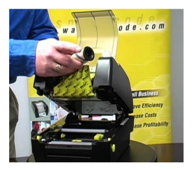
Load the labels centered on the yellow supply spindle, and place the wing guides on either side. Tighten the yellow label sensor/guides so they are snug but do not bind the label stock.
