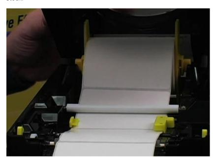
Another view of properly loaded labels and label sensor/guides. The labels lay flat across the top the gray platen roller and metal tear-off bar. The label sensor (yellow guides toward the front) should be snug to the label strip (but not binding).
