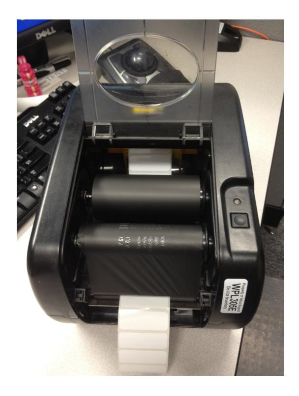
This shows the ribbon loaded properly. The ribbon comes down from the unused supply roll in back, straight across toward the front, then up the front to the used takeup roll. This is also the dull/ink side of the ribbon, which comes in contact with the labels.
