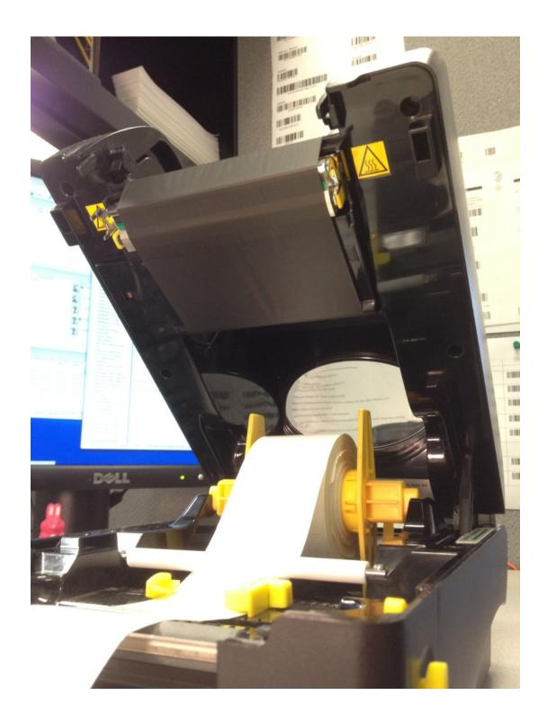
This is the print head. The dark line heats up to transfer the ink from the ribbon to the label (thermal transfer), or to darken the coated labels or tags (ribbonless, direct thermal):
