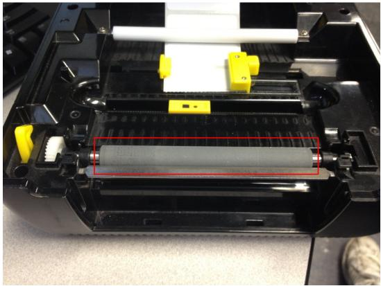
Below is the gap sensor component. The exact location of the sensor is at the + crosshatch
