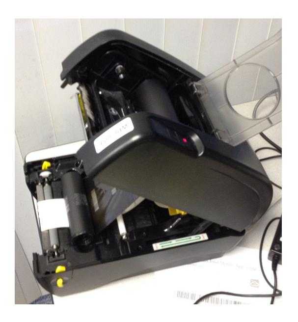
This shows the ribbon loaded properly. The unused supply roll is in back, and the used takeup roll is in front. The dull side is what shows here; this is the ink side of the ribbon. The shiny side does not have ink on it.
