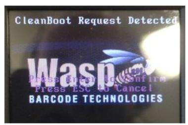
The movie file linked below demonstrates the Warm Boot keypresses, and continues with the Clean Boot's 0+Red Phone to show the confirmation screen (the movie ends here). At this point, press ENT on the keypad to confirm the Clean Boot, or press Red Phone button to cancel.
